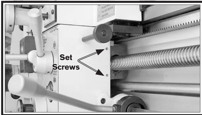
Figure 121. Half nut gib adjustment.
